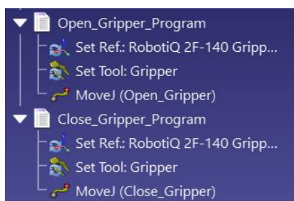
Figure 20.25. The Open_Gripper_Program and the Close_Gripper_Program
