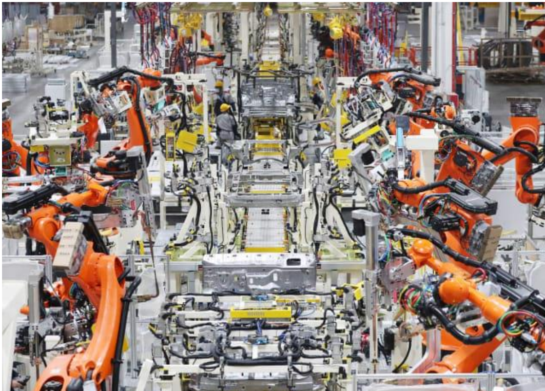
Figure 3.1. Industrial robots are at a car factory.
